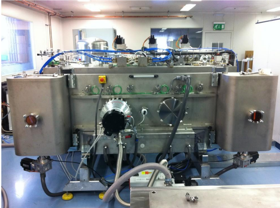
Figure 2 Hybrid sputtering and evaporation prototype based on the CIGS formation process process initially developed by University Milano Bicocca (Sunplugged)
